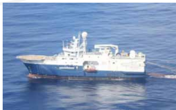
KENYA L8-MBAWA 3D SEISMIC SURVEY-FUGRO GEO BARENTS (8 STREAMER 3D VESSEL)
